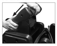
4. Connect the serial cable between the charger and tighten the screws on each connector.
