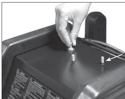
One of three pre-installed bolts for the control module mounting bracket.
