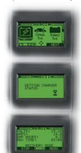
From the main menu, when the diagnostic charging icon is highlighted, the EXP controller shows that the GR8 is in use
